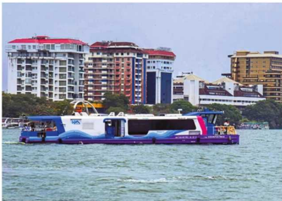
The Kochi fleet operates mostly on lithium-titanium battery technology, with hybrid propulsion as an emergency backup.
